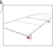
4. Connect feet by pressing and pushing.
