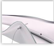
6. Thread cable support through eyelet.
