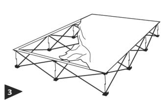
Work in continuous direction around the frame until graphic is completely attached.
