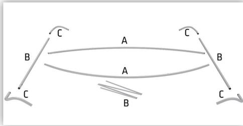
**1** Assemble the two long curved and long straight sections (Connected with bungee cord). The frame is symmetrical. Either curved pole can be top or bottom.
