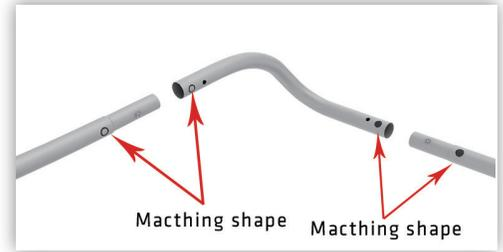
**2** Connect corner sections to curved and straight sections with matching shape codes.
