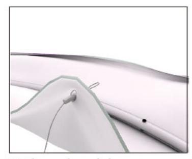
6.Thred cable support through eyelet.
