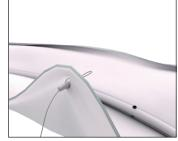
6.Thread cable support through eyelet.
