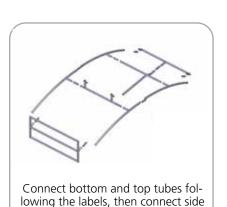
tubes. Note tubes with velcro on face.
