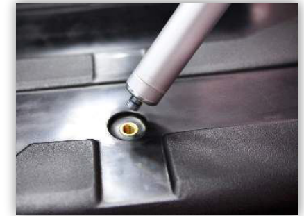
4. Screw the poles into the case
