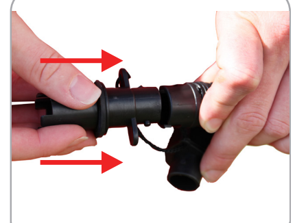
Connect nozzle piece into end of blower hose 4
